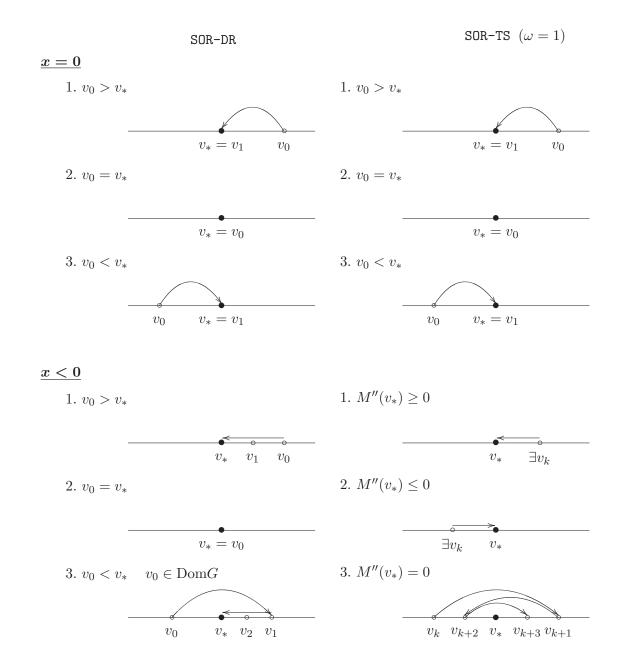
Figure 4. Convergence patterns for the SOR-DR and SOR-TS ( $\omega = 1$ ) algorithms. The left and right half of the figure shows all the possible convergence patterns for the SOR-DR and SOR-TS  $\omega = 1$  algorithms, respectively. The two cases x = 0 and x < 0 are listed separately. The two algorithms are always globally well-defined, except that when  $v_0 < v_*$  and x < 0, we need  $G(v_0)$  to be well-defined to guarantee that  $\{v_k\}$  is defined.
