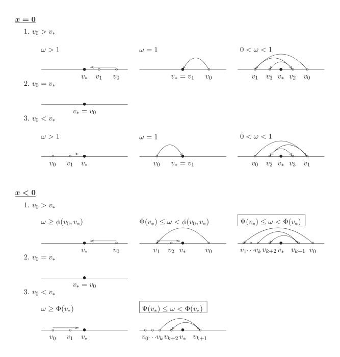
Figure 3. Convergence patterns for the SOR algorithm. This figure shows all the possible convergence patterns for the SOR algorithm. The two cases x = 0 and x < 0 are listed separately. Except for the two cases whose conditions are boxed, all the conditions above each subplots are both sufficient and necessary for each particular convergence pattern to occur. The two boxed conditions are only necessary conditions.
