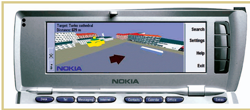
Figure 2. The TellMaris client application interface lets users navigate a 3D model of their location and discover nearby landmarks and services.
