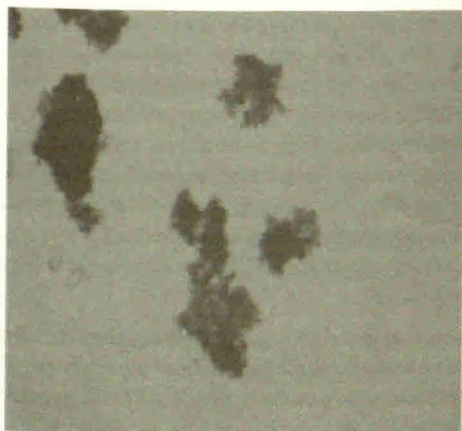
Figure 5: An image of MWNT alone taken with a light microscope at 40X optical zoom. Shows isolated MWNT clusters in solution
