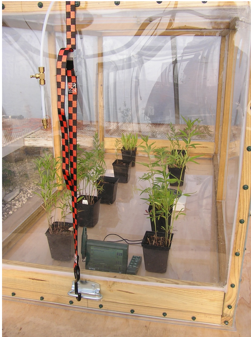
Fig 2.1. Experimental exposure chambers with chamber covers raised by a pulley system and treatment plants in place in the center of individual cells on the chamber floor grid.
