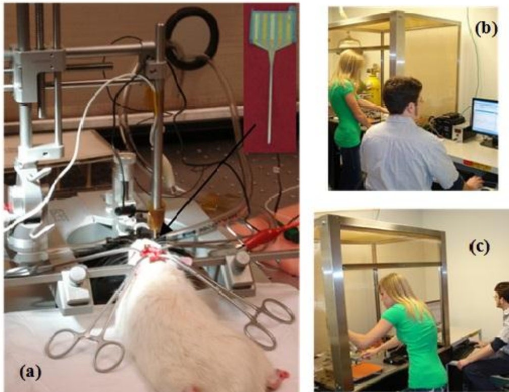
FIGURE 4: (A) ANIMAL SUBJECT ON THE SURGICAL WORK STATION WITH THE NEURAL PROBE, INDICATED BY AN ARROW, MOUNTED ON A STEROTACTIC FRAME. (B) / (C) LAUREN KEGLEY AND PHILLIP HANKINS CALIBRATING THE DATA ACQUISITION SYSTEM TO PREPARE FOR A LIVE ANIMAL EXPERIMENT.
