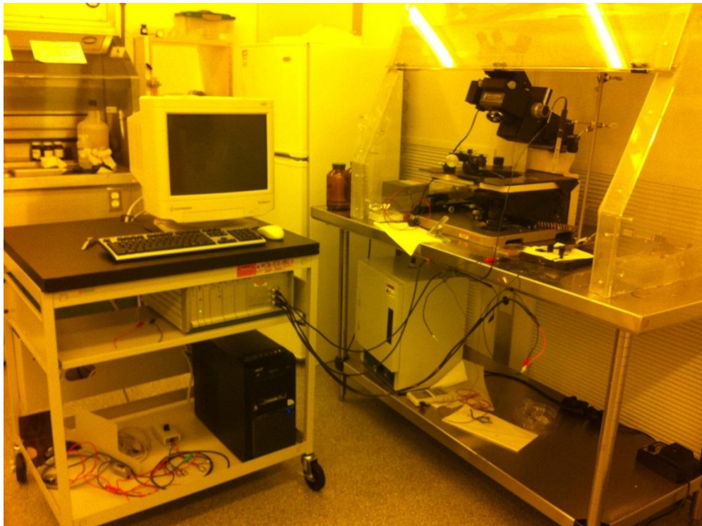
FIGURE 5: IMPEDANCE TESTING SETUP IN THE INNOVATIVE NANO- AND BIO- DEVICES LABORATORY CLASS 100 CLEAN ROOM.
