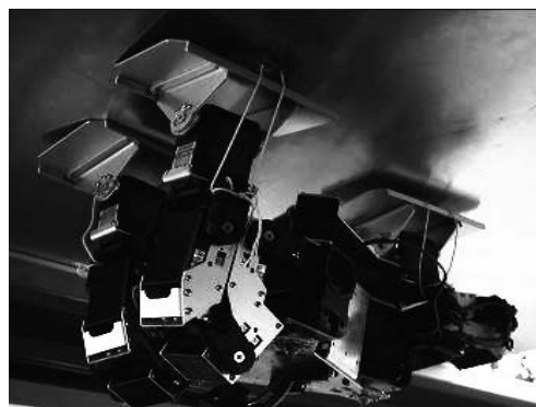
Fig. 1: The inverted walking on the roof by using the suckers.
