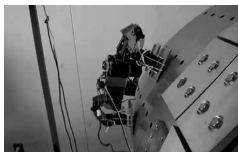
Fig. 2: The TLR climbing up the curved wall.
