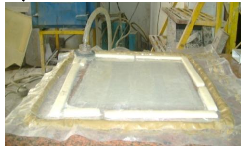
Fig – 2 vacuum bagging process
