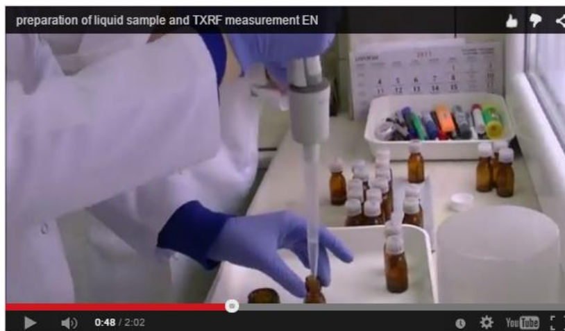
Figure A.4 A screenshot of the video instruction concerning “sample preparation and measurement” which shows the sample treatment for measurement with the TXRF technique.
