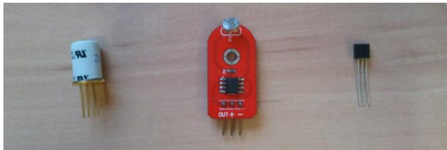
Figure 3: Carbon monoxide (CO), luminosity and temperature sensors
