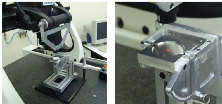
Fig. 2. Views of the CMM, the sensor, the fixture and the test surface during a scanning operation
