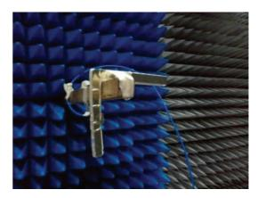
FIGURE 19: Antenna prototype mounted on the rotating platform for radiation pattern measurements.
