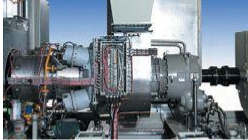
Figure 3.1: A simple-cycle gas turbine that generates 1.9 MW of shaft output power (OPRA Gas Turbines)
