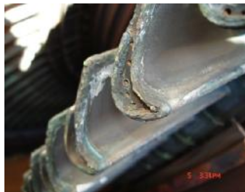
Figure4.5: Corrosion due to fuel potassium content effect on blades
