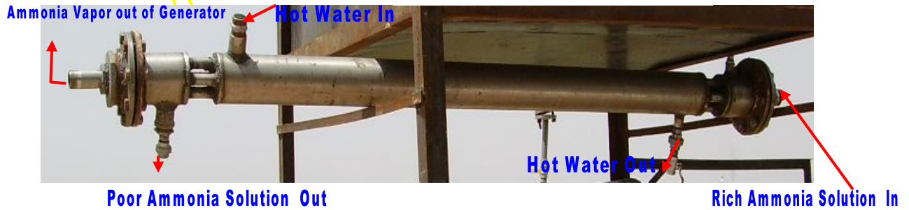
Fig. 4.14 Shell and Tube Heat Exchanger
