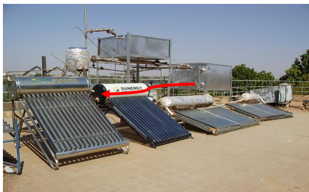
Fig. 4.33 Connection of Outlet Tube of Double Heat Exchanger to Evacuated Collector
