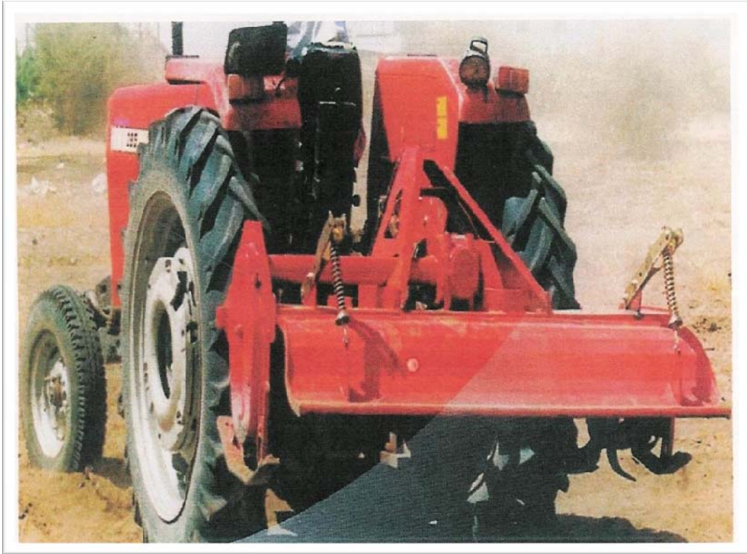
Fig (3-3-5) shows hitching of rotary hoe
