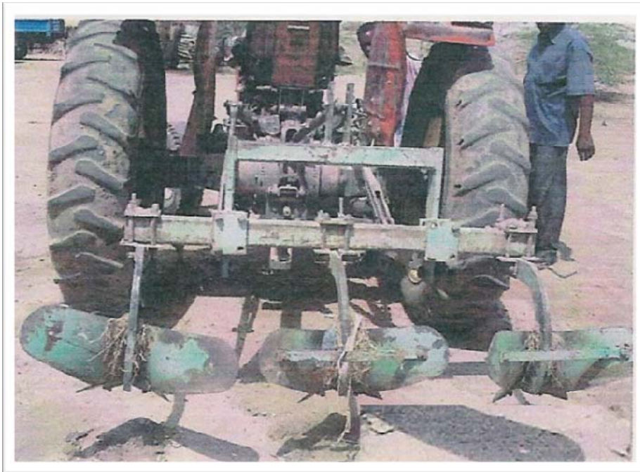
Fig (3-3-4) shows the hitching of ridger
