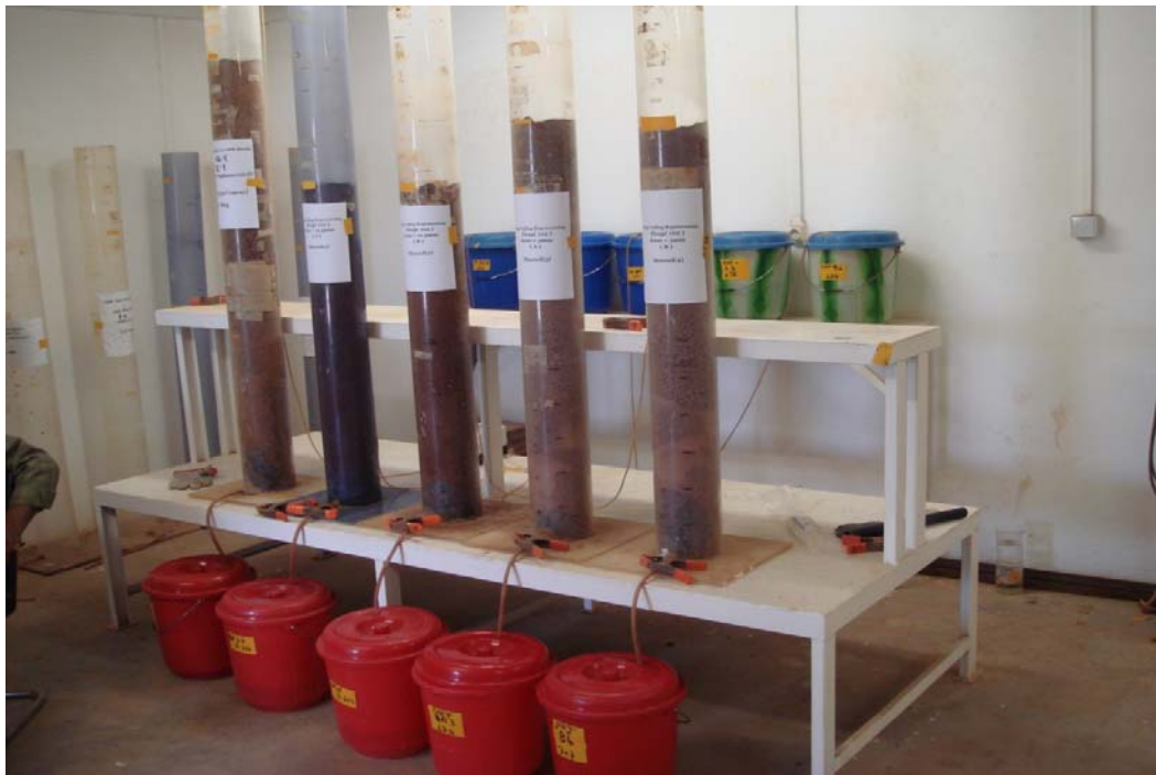
Fig.5.8. Percolation leach test [column test] in Lab-size
