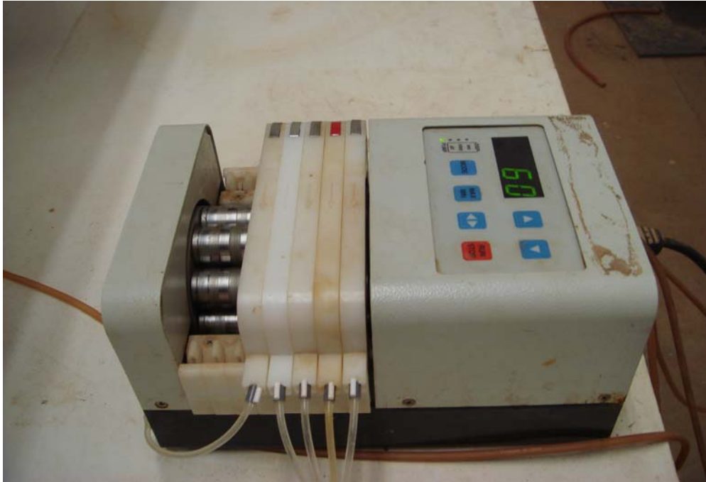
Fig.5.9 Pump used to spray the inlet solution to the in to the column
