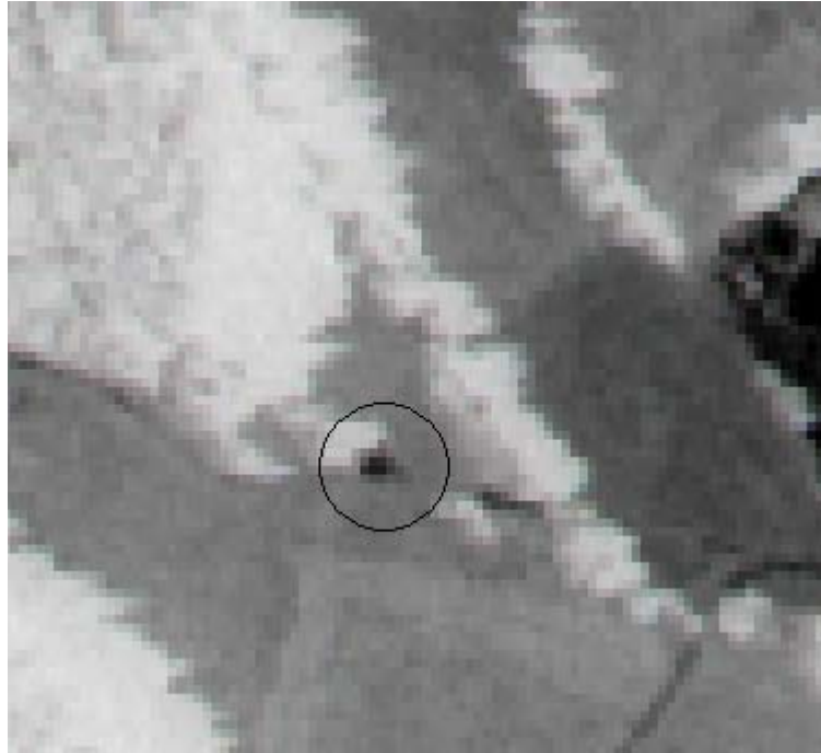
Figure (8.19) A typical control point with 30 \mu m pixel size.
