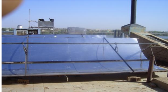
Fig (1). The developed trough model
