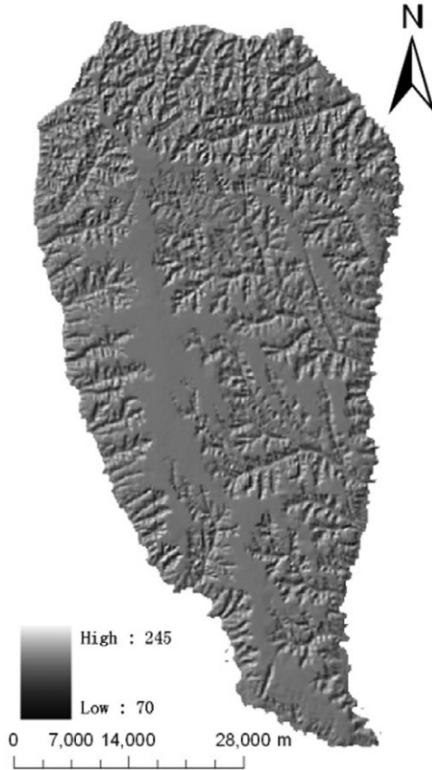
Figure 3 Shaded relief map in 3D of Dong-Zhi tableland simulated after the refinement process is stopped (Light from 135° with a dip angle of 45°)
