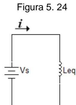
$$\begin{aligned}v_s &= v_1 + v_2 + \cdots + v_N \\&= L_1 \frac{di}{dt} + L_2 \frac{di}{dt} + \cdots + L_N \frac{di}{dt} \\&= (L_1 + L_2 + \cdots + L_N) \frac{di}{dt}\end{aligned}$$
