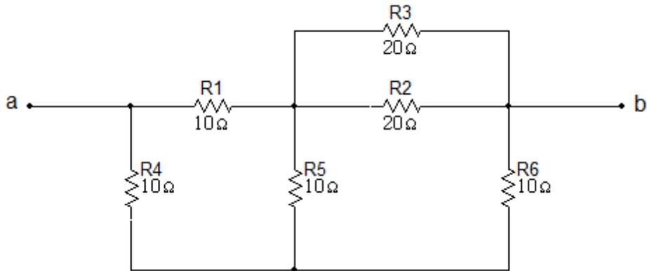
$$R_7 = R_3 \parallel R_2 = \frac{20 \times 20}{40}$$
