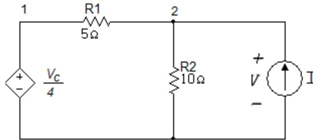
$$I = \frac{V_2}{10} + \frac{V_2 - V_1}{5}$$
