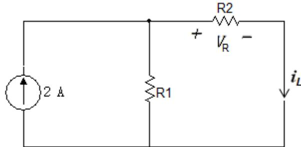
$$i_L(0^-) = i_L(0^+) = 2A \left( \frac{R_1}{R_1 + R_2} \right)$$
