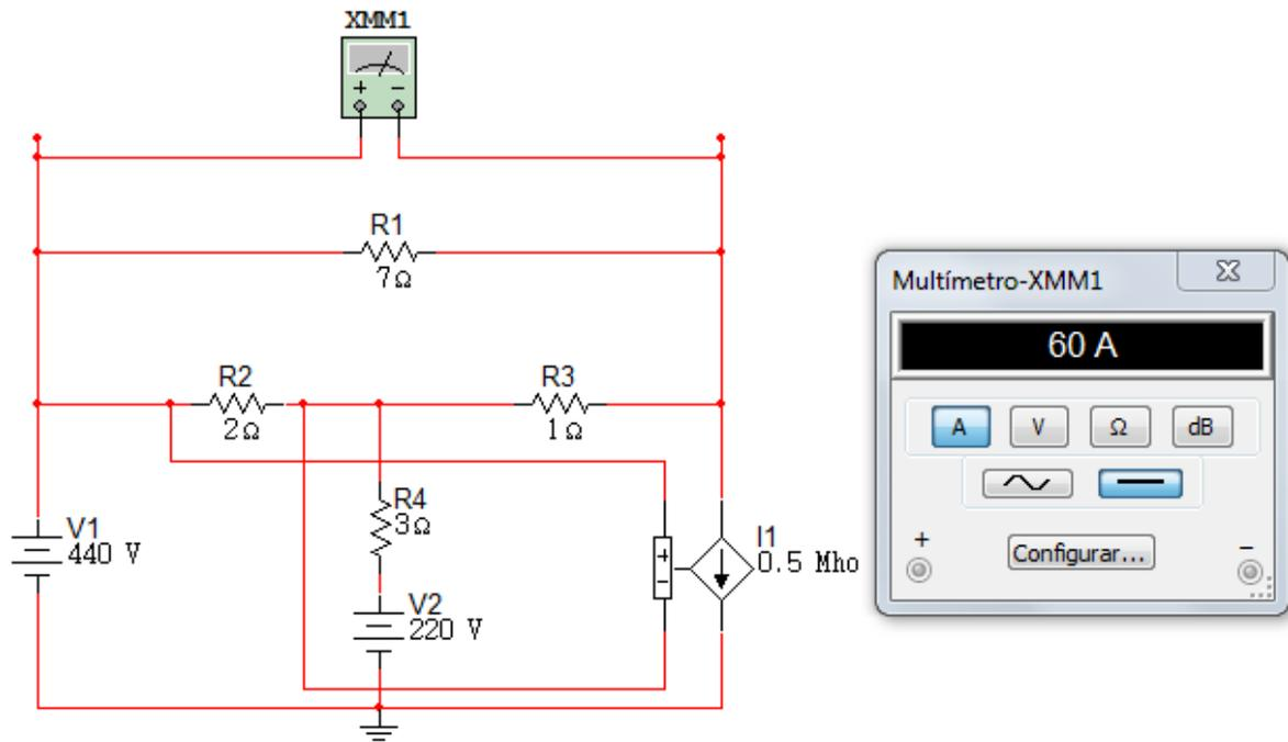
$$R_{th} = \frac{V_{th}}{i_{sc}} = \frac{184.8V}{60A}$$
