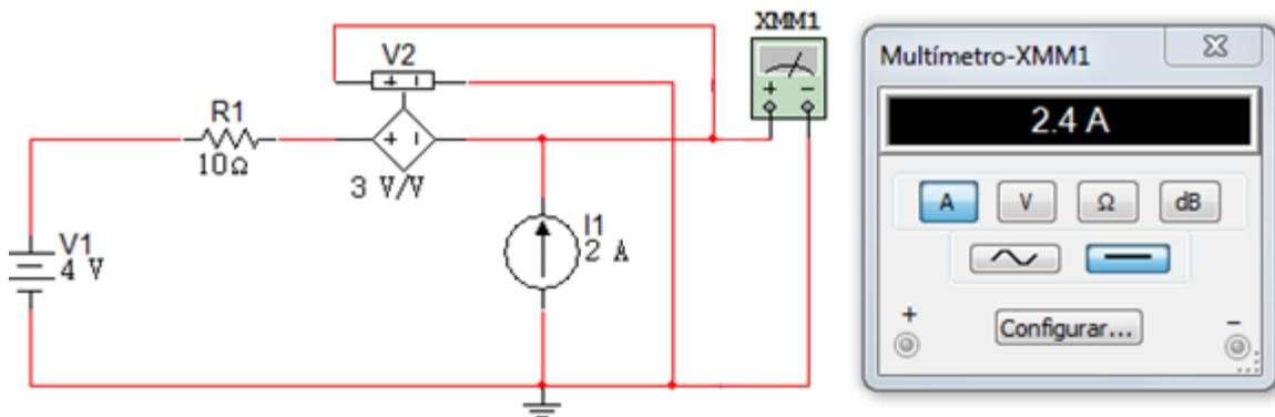
$$R_{th} = \frac{V_{th}}{I_{sc}} = \frac{6V}{2.4A}$$
