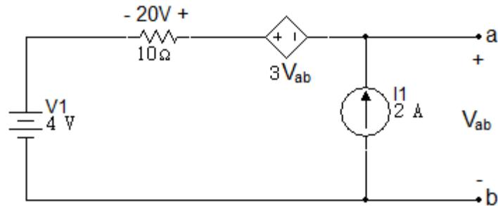
$$V_{10\Omega} = (2A)(10\Omega)$$
