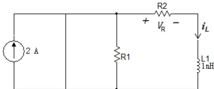
$$i_L(t) = \frac{2R_1}{R_1 + R_2} e^{-\frac{R_2}{20 \times 10^{-3}} t} = \frac{2R_1}{R_1 + R_2} e^{-50R_2 t}$$
