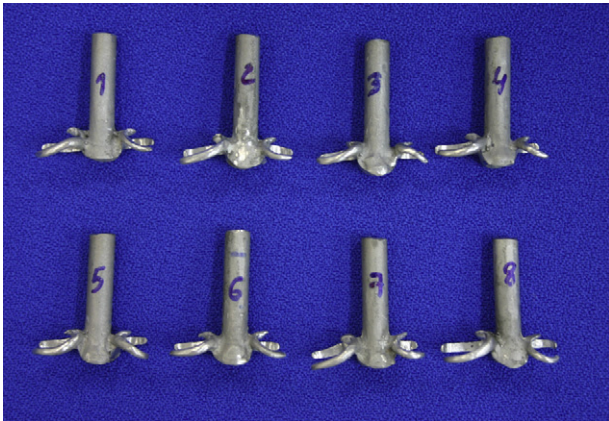
Fig. 2. View of specimens entirely made in Co–Cr.
