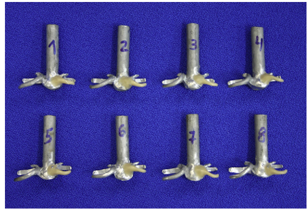
Fig. 3. View of specimens with anterior retentive arm made in acetyl resin.
