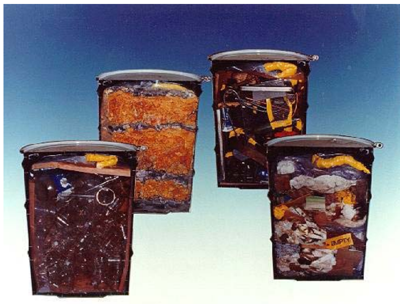
Figure G5-1. Legacy TRU wastes packaged in 55-gallon drums with and without liners, bags, and stabilizing sorbent media.
