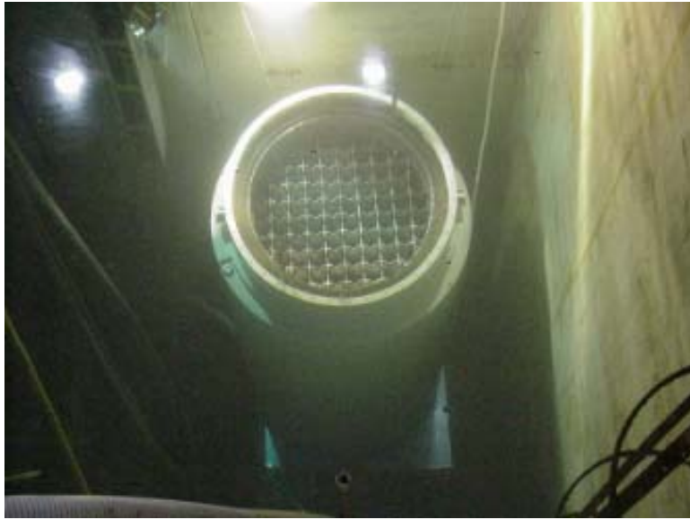
Figure G2-2. Holtec International cask in fuel storage pool). Figure copied from Holtec International Web site.
