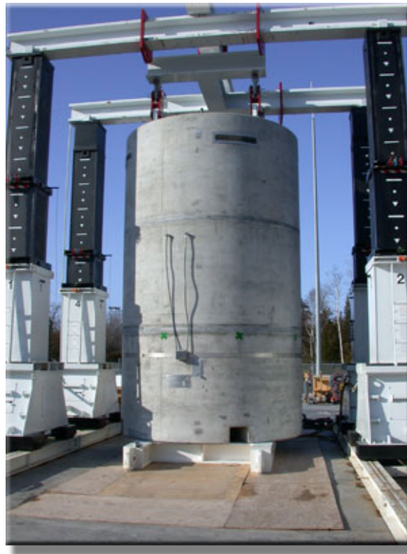
Figure G2-5. BNG Fuel Solutions vertical cask lift. Figure copied from BNG Web site.
