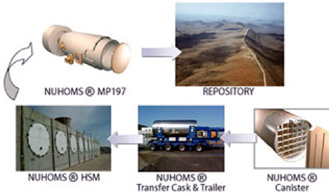
Figure G2-4. Transnuclear NUHOMS design (Note horizontal storage allowing stacking). 9
