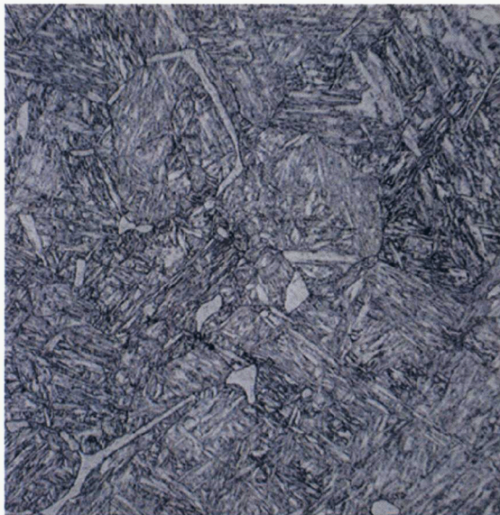
#29 9Cr-2WVTa 1100°C/700°C 200X 20µm 50H 2 O/5HNO 3 /1HF
