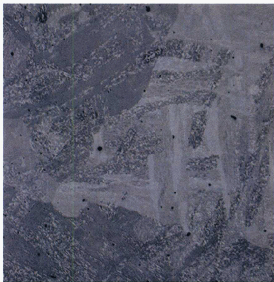
3Cr-3WV #1 1050°C Long. View 50X 100μm 5CH 2 O/5HNO 3 /1HF
