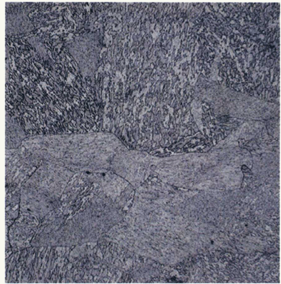
#2 3Cr-3WVTa 1100°C/750°C 200X 20µm 50H 2 O/5HNO 3 /1HF
