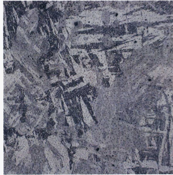
3Cr-3WVTa B #21 1100°C Long. View 50X 100µm 50H 2 O/5HNO 3 /1HF
