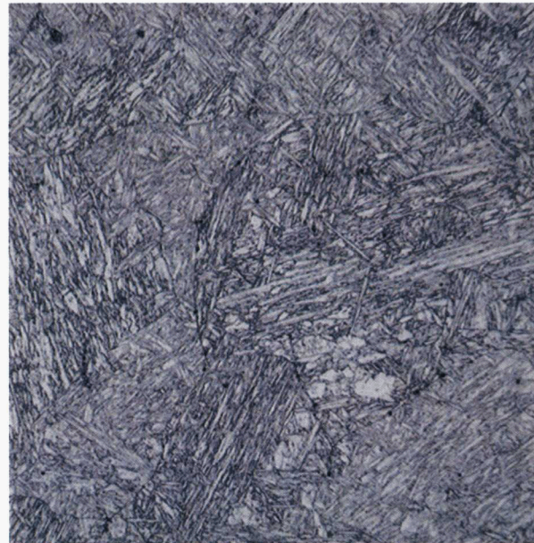
#45 COST CB2 1100°C/700°C 200X 20µm 50H 2 O/5HNO 3 /1HF
