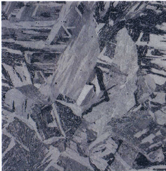
3Cr-2WMoVTa #3 1100°C Long. View 50X 100µm 50H 2 O/5HNO 3 /1HF
