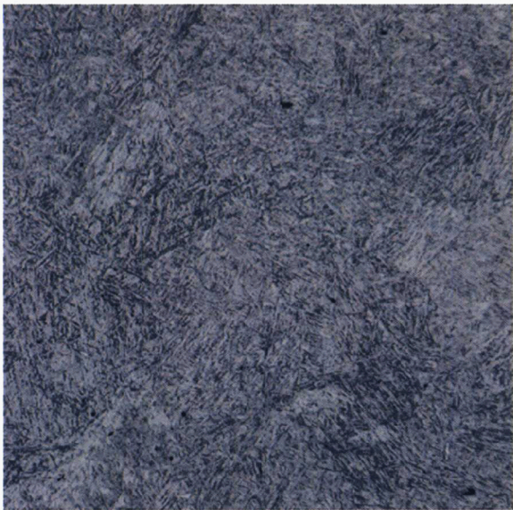
11Cr-2WVTa #31 1100°C Long. View 50X 100μm 50H 2 O/5HNO 3 /1HF
