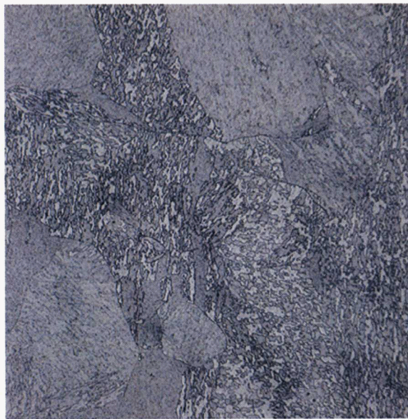
#1 3Cr-3WV 1100°C/700°C 200X 20µm 50H 2 O/5HNO 3 /1HF
