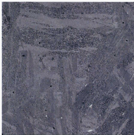
3Cr-3WV Ta #2 1050°C Long. View 50X 100μm 50H 2 O/5HNO 3 /1HF
