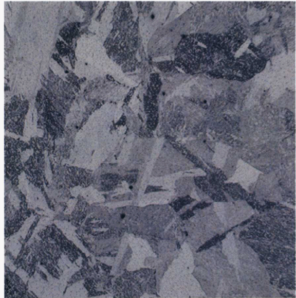
3Cr-3WV Ta #2 1100°C Long. View 50X 100µm 50H 2 O/5HNO 3 /1HF
