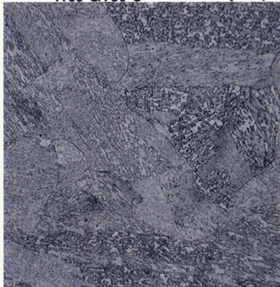
#3 3Cr-2WMoVTa 1100°C/750°C 200X 20µm 50H 2 O/5HNO 3 /1HF
