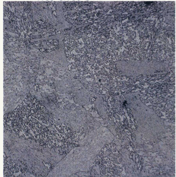
#21 3Cr-3WVTaB 1100°C/750°C 200X 20µm 50H 2 O/5HNO 3 /1HF
