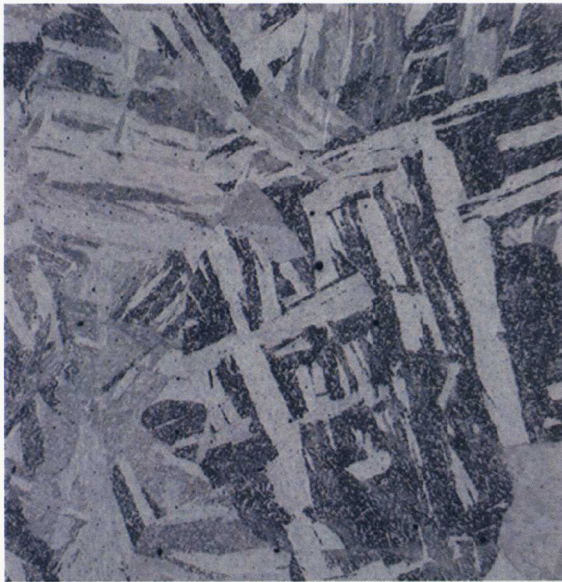
3Cr-3WV #1 1100°C Long. View 50X 100µm 50H 2 O/5HNO 3 /1HF
