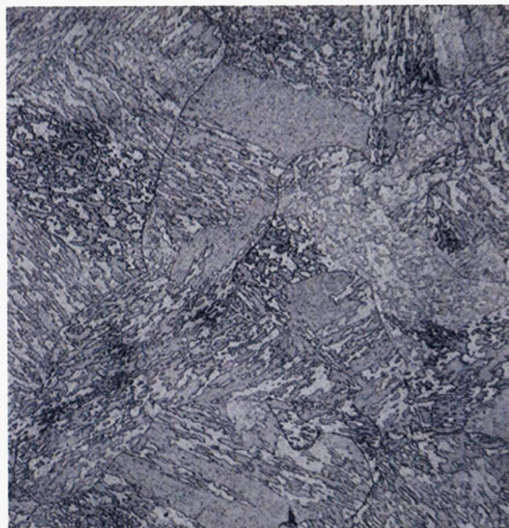
#3 3Cr-2WMoVTa 1100°C/700°C 200X 20µm 50H 2 O/5HNO 3 /1HF
