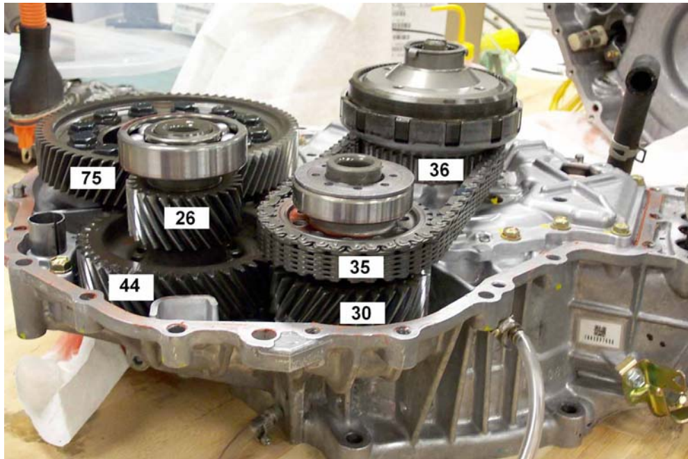
Fig. 2.6. 2004 Prius gears with number of gear teeth shown.
