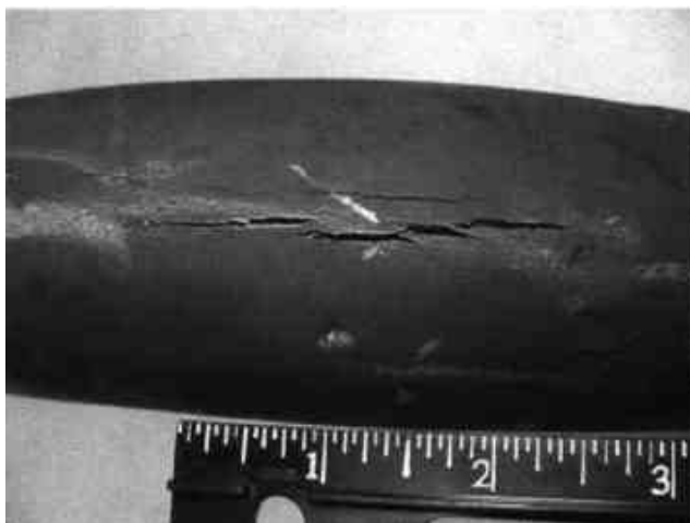
Figure 3.48. Failure of superheater tubes of T91 steel due to improper intercritical heat treatment. Tubes were in service for only four years [Henry 2005].
