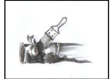
FIGURE 5C: SOAKING IT IN BITUMEN FOR 24 HOURS
