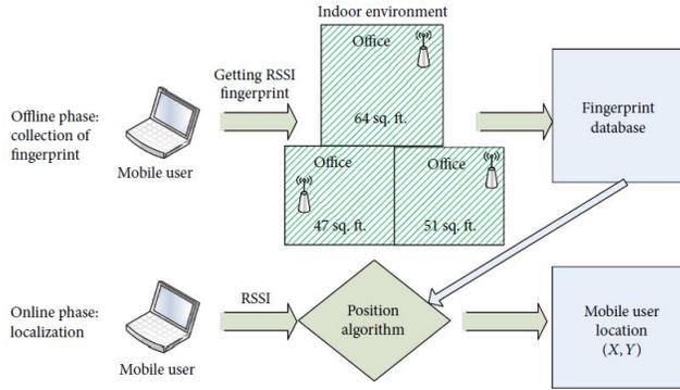
FIGURE 2.7. Positioning using a fingerprinting system
