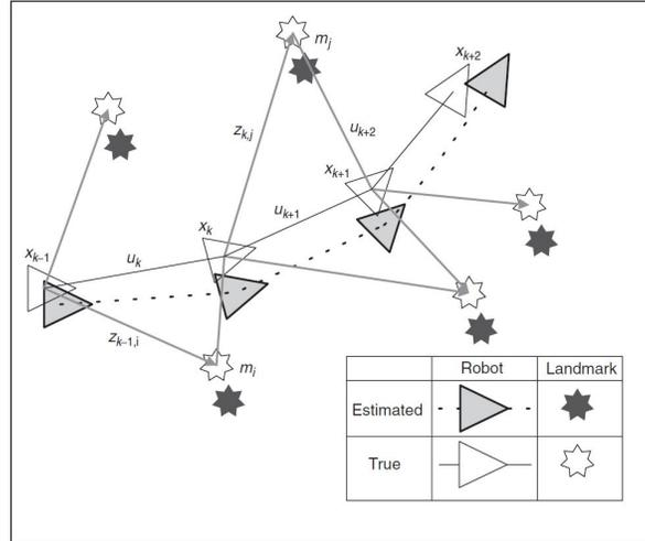
FIGURE 5.1. SLAM using landmarks
