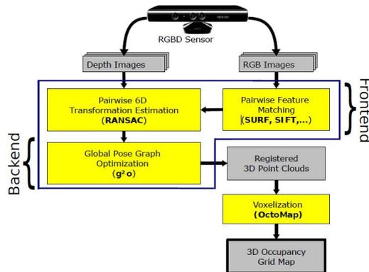
FIGURE 5.2. Schematic overview of RGBD SLAM
