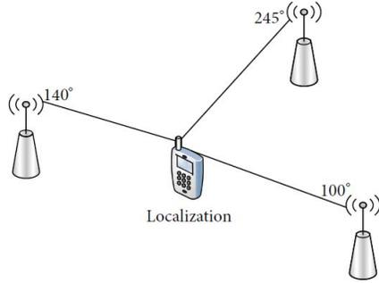
FIGURE 2.10. Calculation of position using AOA
