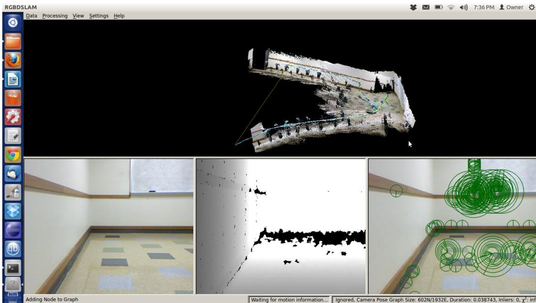
FIGURE 5.8. 3D modeling of a room at the electrical engineering department
