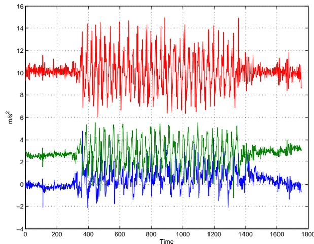
FIGURE 4.4. Change of acceleration in the X,Y and Z axes when movement is detected
