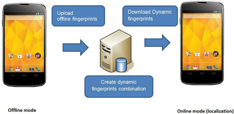
FIGURE 4.18. Android applications and server interaction
