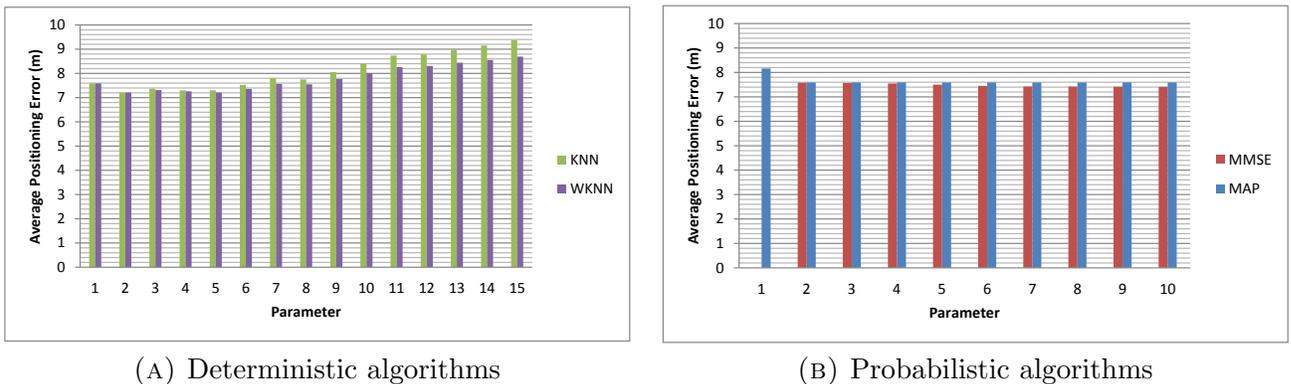
FIGURE 4.22. Average positioning error of the non-dynamic IPS
