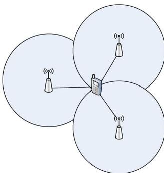
FIGURE 2.8. Calculation of position using TOA
