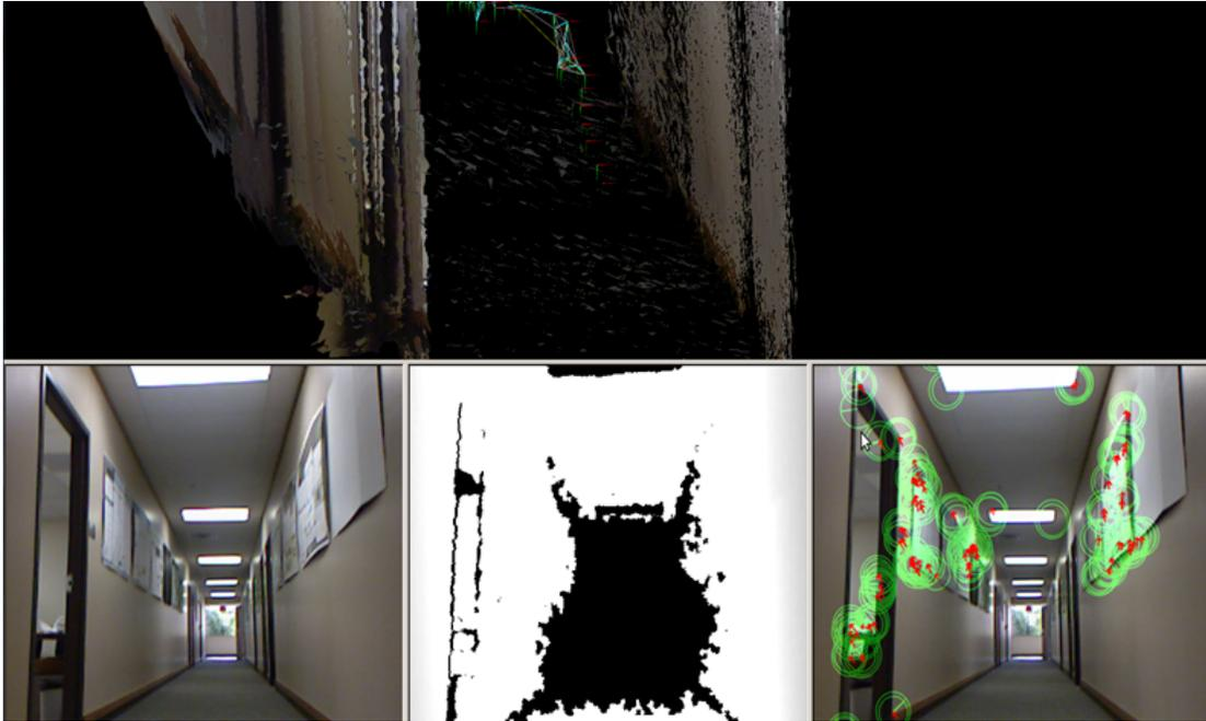
FIGURE 5.5. Extraction of visual features that are associated to 3D points
