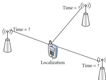
FIGURE 2.9. Calculation of position using TDOA
