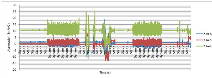
FIGURE 4.6. Acceleration signals from user movement pattern for experiment 1
