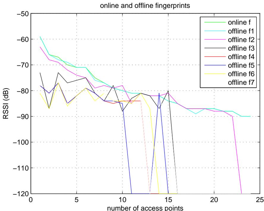
FIGURE 3.3. RSSI levels from 7 fingerprints
