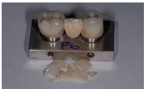
Fig. 2. Partial fracture of the porcelain layer of a specimen from the Procera group.
