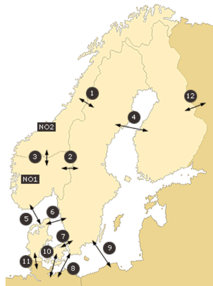
Figure 9: Different zones of Nordpool to which market splitting is applied. Connection 1 between Northern Norway NO2 and Sweden represents the two-node model and is frequently constrained. it represents a two-node model with the major interconnection to Sweden by transmission links
