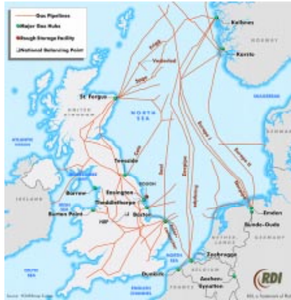
Figure 1: Gas Pipelines Northern Europe (Copyright Platts, 2001)
