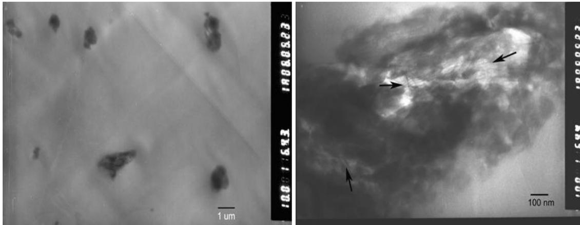
Fig. 3. TEM for the PET-co-DDP/ZrP nanocomposite
