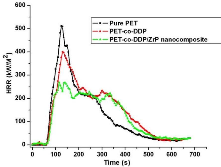
Fig. 5 Heat Release Rate (HRR) for samples
