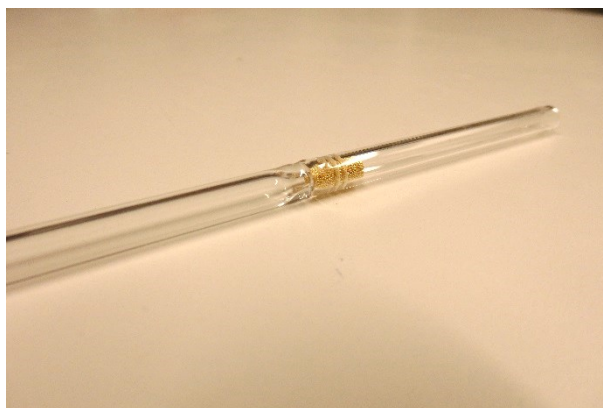
Figure 4. Picture of a gold cartridge from Tekran Instruments Cooperation © used for collecting GEM/TGM in air.
