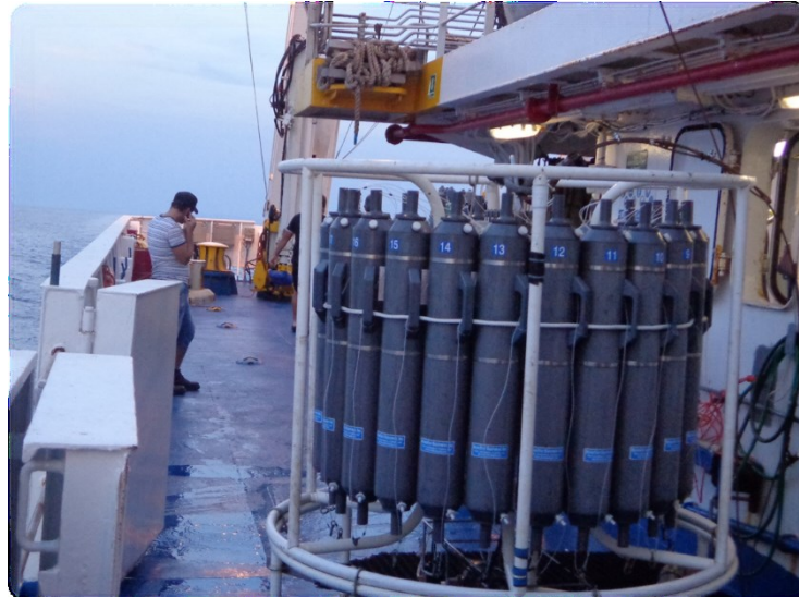
Figure 8. A CTD/Rosette system used to sample seawater obtaining deep water profiles of DGM concentrations. The system on the picture was used during the Fenice 2011 and Fenice 2012 campaigns.
