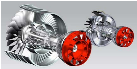
Fig. 4: Turbine Rear Structures on different size engines
