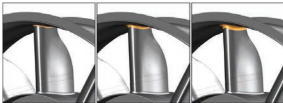
Fig. 8: Blend radius set to vary between 2.5mm and 10mm
