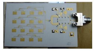
Fig. 3.3. Photo of the 24 GHz SOM with integrated 4×4 patch array antenna.
