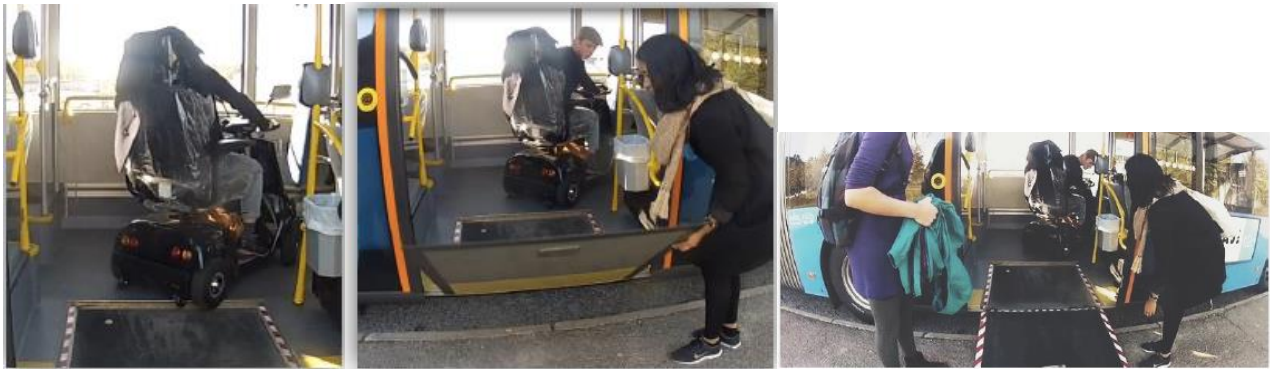
Figure 3 Student project in Gothenburg city testing how busses are adapted for wheel-chairs. The ramp needs to be fold manually and there is limited space for the wheel-chair inside the bus. The wheel-chair driver needs to have an assistant or get help from the driver. The loading/un-loading procedure affects the time schedule of the bus.
