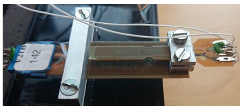
Figure 3. Built prototype I with MIDE v21b at the bottom, the coupling fixture and the MIDE v22b at the top.
