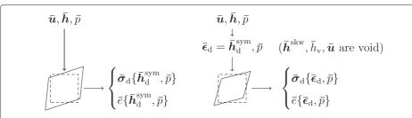
**Figure 3 Comparison of the RVE-problem formulations.** Original formulation (left) and Canonical formulation (right).
