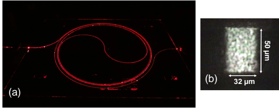
Fig. 1: Images of (a) the spiral waveguide illuminated with red light and (b) the waveguide output facet illuminated with 850 nm light.
