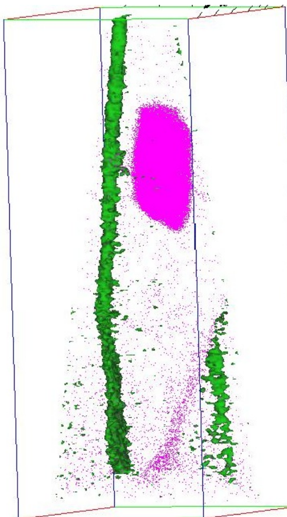
Figure 1: Iso-concentration surface of 3.2 at% Sn (green) displayed to show retention to a crystallographic pole in the metal of an LK3 sample. The presence of Fe in an SPP as well as grain boundary segregation of Fe is also rendered (purple). Size of the box is 250x100x100 nm 3 .
