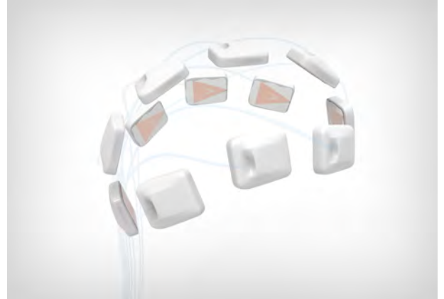
Figure 1. The 3-d distribution of the isosceles triangle patch antennas
