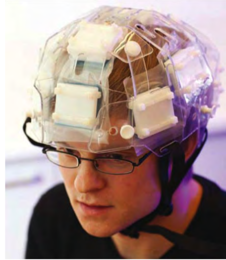
Figure 7. The second prototype system, in which the 12 patch antennas have been mounted on a custom built supporting structure.
