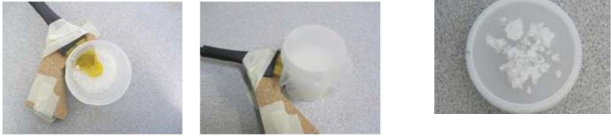
FIG 4. Left: probe inserted in the cup. Middle: the cup sealed with Parafilm. Right: granules of PCM (photo B. Seng)
