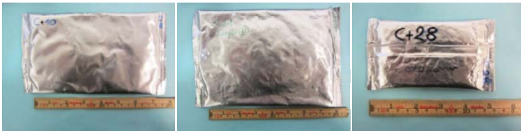
FIG 1. Pouches with ClimSel 10, ClimSel 21 and ClimSel 28 in laboratory environment at 21 °C. (photo B. Seng). Notations ClimSel 10, ClimSel 21 and ClimSel 28 stand for salt hydrates with melting temperatures at 10 °C, 21 °C and 28 °C respectively.
