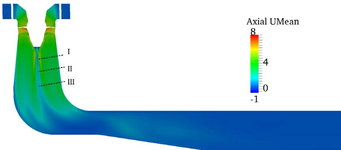
Figure 2. Mean axial velocity [ m/s ] at the center plane. The experimental data is available at cross-sections I, II and III.
