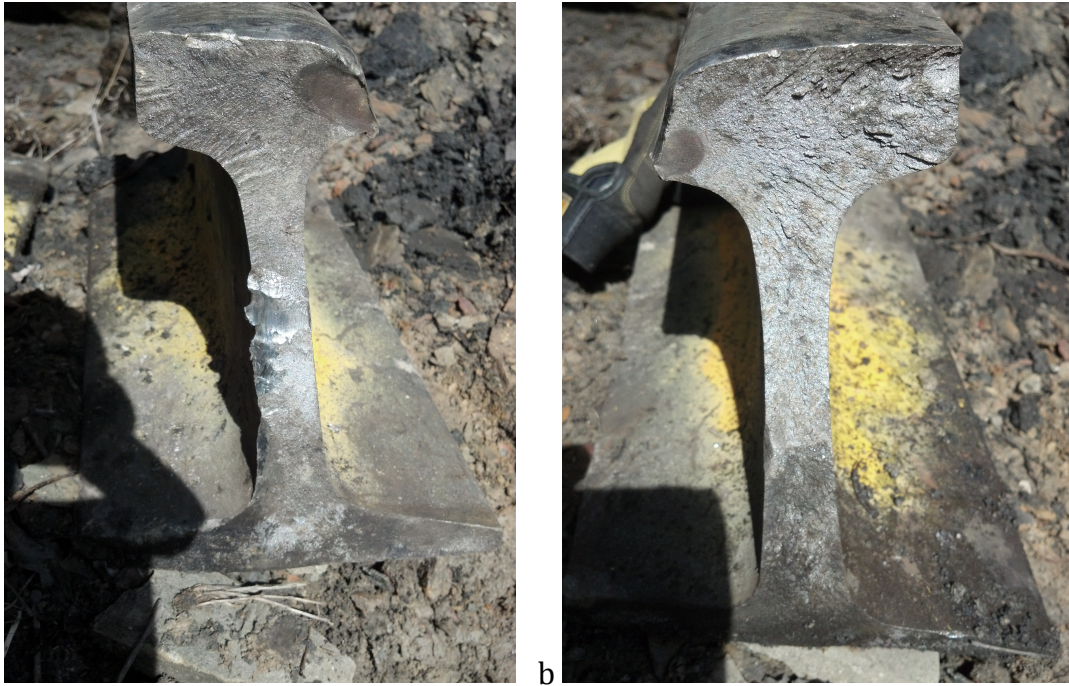
Figure 11 Fractures at sections 1HiC (a) and 1HiD (b)
