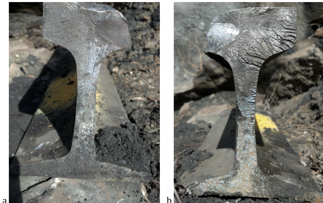
Figure 10 Fractures at sections 1HiA (a) and 1HiB (b)
