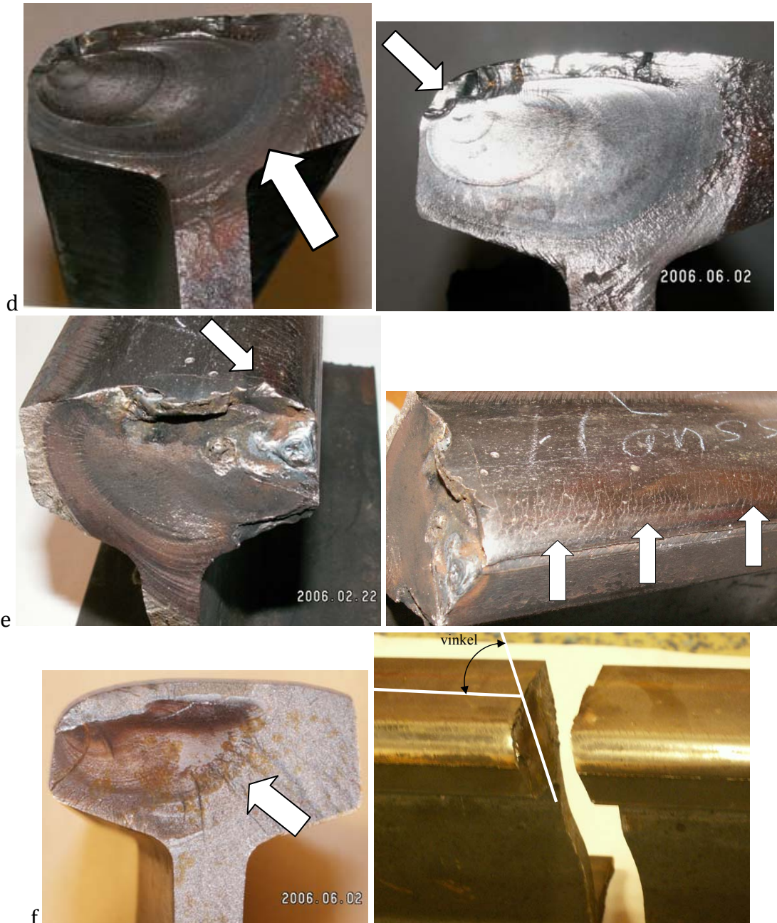
Figure 7 Fractures surfaces of the investigated rail sections b–f as detailed above.
