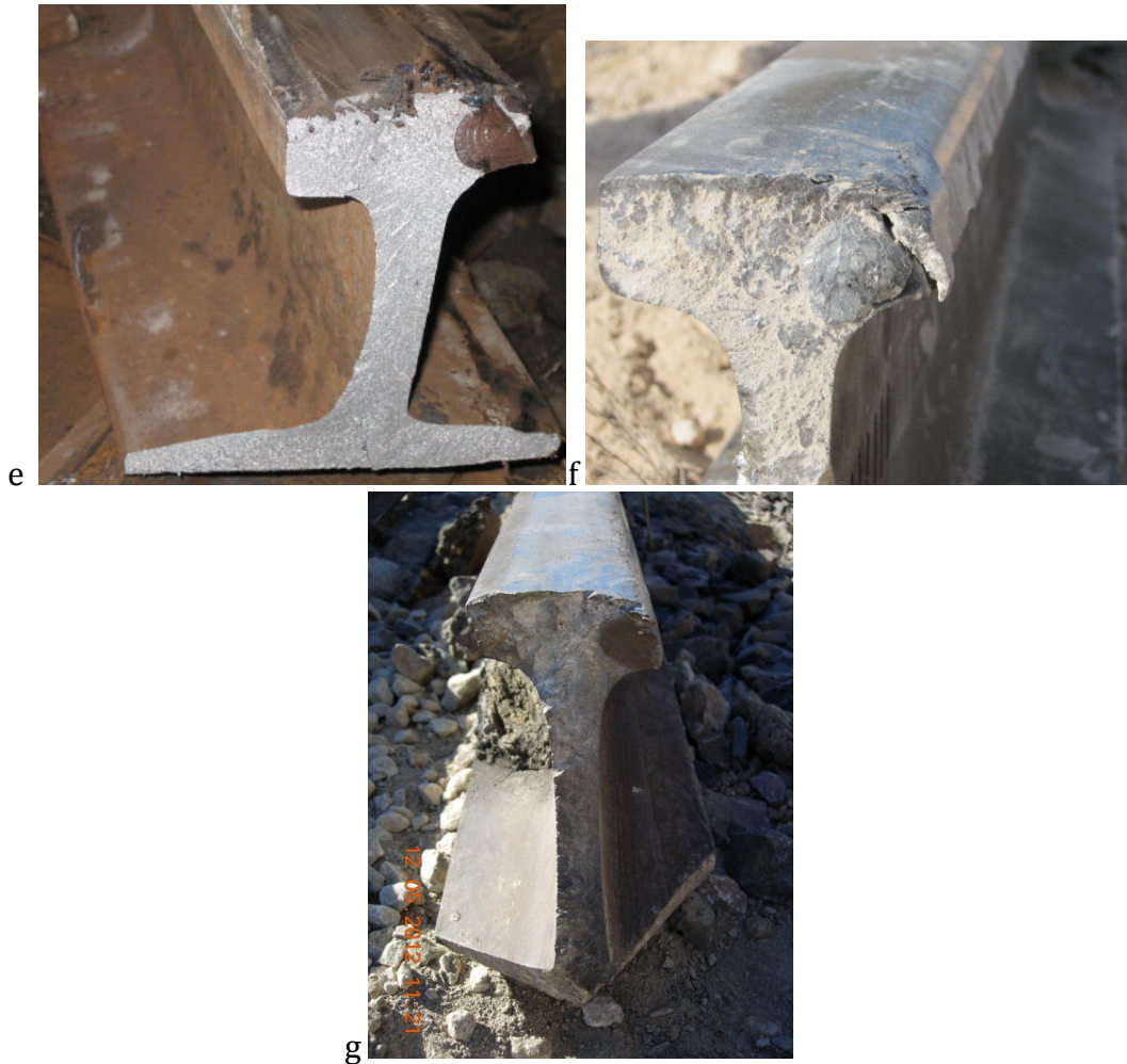
Figure 13 Overview of fractured rails
