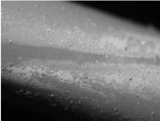
Figure 6 Surface degradation for a wire exposed to 8 Mcycles of PWM waveform with smoothness level 1 and amplitude 2.5 kV pp . Note that the surface outside the contact area is severely more damaged than for the higher smoothness, shown in figure 7.
