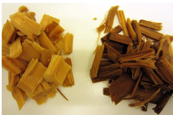
Figure 6.6 Steam-exploded wood chips from the bench-scale equipment. Left: chips exploded at four bar. Right: chips exploded at seven bar.
