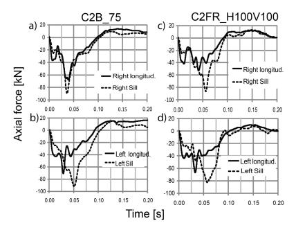
Figure 18: Axial loads measured in the right [(a) and (c)] and left [(b) and (d)] longitudinal structures of the car when crashed against FWRB [(a) and (b)] and against e.a. FUPD (c)
