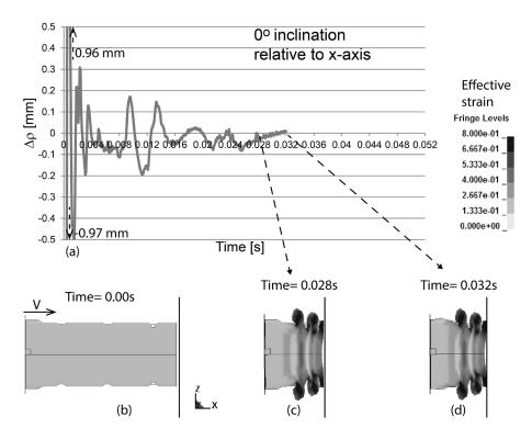
Figure 13: Crash body  $1 - 0^{\circ}$  inclination relative to x-axis. (a) RED curve, (b) initial state just before impact, and states at approximate time points when (c) the buckling stops and (d) displacement reaches its maximum value, respectively at lower row with effective strain fringe pattern.
