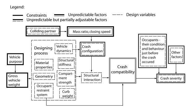
Figure 17: Model of parameters and interactions influencing compatibility
