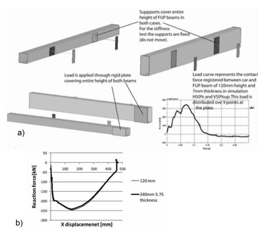
Figure 9: *a)* Set-up of the bending test simulation with a loading curve; *b)* Displacement of the FUPD cross-beam end for the different cross-beam heights under bending test
