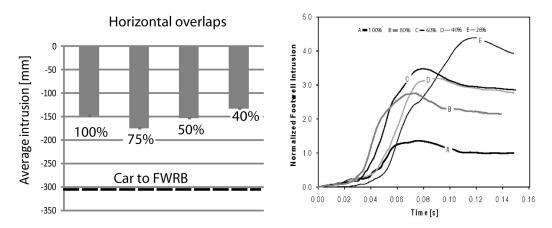
Figure 8: a) Average intrusions from car to e.a. FUPD for different horizontal overlaps in comparison to intrusions caused by impact into FWRB b) Normalized (to intrusions for full overlap) footwell intrusions from car-to-car simulations for different horizontal overlaps (complementary Paper 1)
