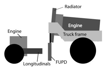
Figure 6: Proposed modification of front truck design
