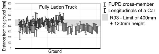
Figure 5: A graphical presentation of relative position between car longitudinals and FUPD crossbeam for fully laden trucks based on the geometrical database
