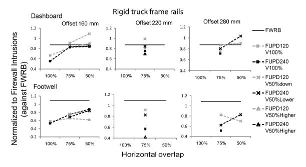
Figure 11: Calculated intrusions of the dashboard and footwell of the car impacting the truck with rigid frame rails
