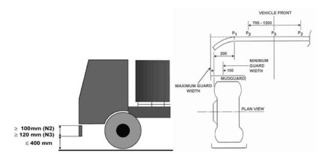
Figure 3: Regulation 93 – Dimension limits and forces that FUPD has to sustained in the static component test.
