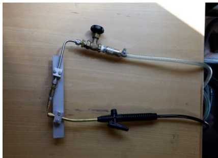
Device for manufacturing of glaze ice using separate nozzles for water and air. Glaze ice sample.
