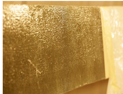
Device for manufacturing of glaze ice using separate nozzles for water and air. Glaze ice sample.
