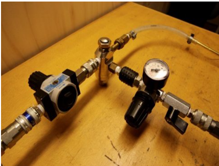
Device for manufacturing of rime ice using one nozzle and mixing of water and air inside. Rime ice sample.
