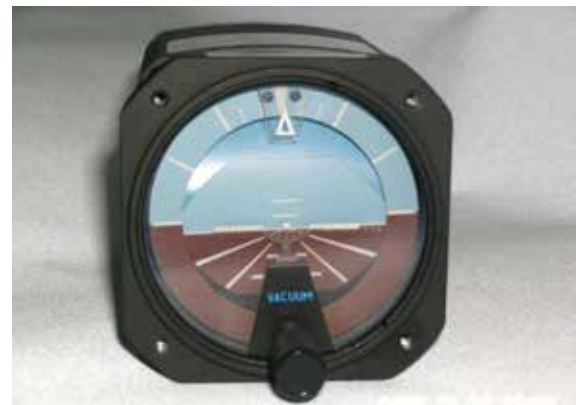
Figure 2. A flight gyroscope showing roll, and pitch. A proposed vessel gyroscope can be used to transmit some "ship sense" to the remote officer of the watch.
