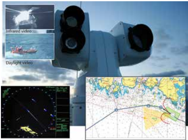
Figure 3: Three tools deliver the bulk of situation awareness to the remote operator: a camera system (top), radars (bottom left) and the electronic chart with AIS information and predicted maneuverability parameters (bottom right).
