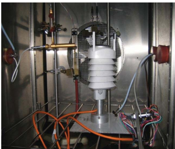
FIGURE 2. Laboratory calibration of weather station at INRiM
