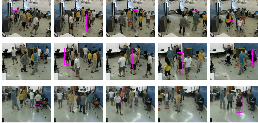
Figure 13: Proposed tracker: tracking results on videos in Case-f. Videos are obtained from views 1-3 of TU Graz Multi-Camera dataset, where an object experiences frequent intersections. Tracked boxes are marked in images (magenta). Row 1-3: results in views 1-3. Key frames (# 3201, 3272, 3369, 3702, 3835) in the video are selected (zoomed in for better inspection of target objects).
