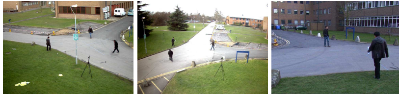
Figure 1.1: Example of a three-camera case with overlapping fields of view, where a dominating ground plane is present [61].
