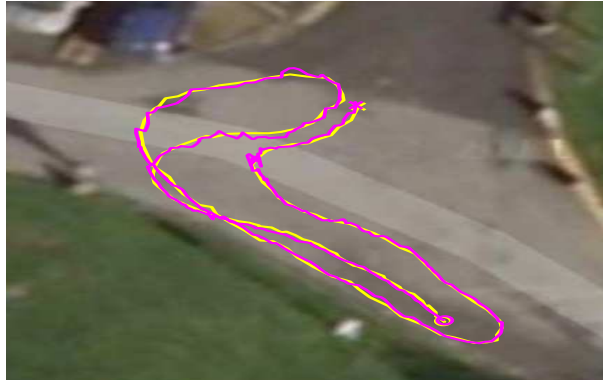
Figure 10: Proposed tracker: trajectories of tracked moving object on video PETS'09 S2.L1: test results and ground truth. The trajectory of tracked object on the ground plane (from the top view) through planer homography mapping. Magenta: from the proposed tracker in View 2. Yellow: ground truth trajectory. 'x' and 'o': starting and end points.
