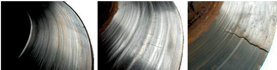
Figure 3 Example of wear (left), heat crazing (middle) and heat cracking (right) [7].
